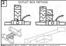
Warning-Risk of fire, electric shock, or personal injury. The fan in this box may be either directly supported from a structural framing member of a building and/or may be mounted to an outlet box marked acceptable for fan support of 31.8 kg(70lbs) or less. Most outlet boxes commonly used for the support of luminaires may not be acceptable for fan support and may need to be replaced. Consult a qualified electrician if in doubt.
